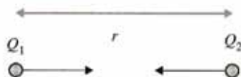
Figure 1.8 The force between two point electric charges is given by Coulomb's law. Shown here is the case of opposite charges.
