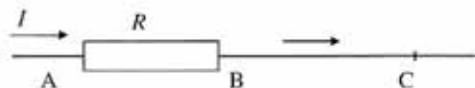
Figure 4.7 There is a potential difference across points A and B but not between B and C.
