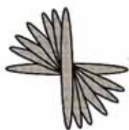
Figure 9.13 The liquid crystal molecules are long and attract each other weakly. Here they form a line that gradually twists as we move into the plane of the page. The orientation of the molecules eventually becomes horizontal at the back plate.
