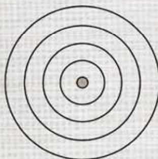
Figure 5.1 The wavefronts emitted by a stationary source are concentric. The common centre is the position of the source.
