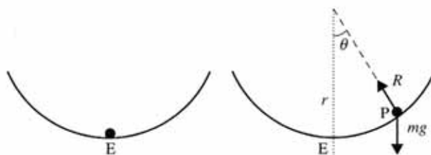
Figure 1.5 A particle in a bowl. The equilibrium position E is at the bottom of the bowl. The particle is released from P.
