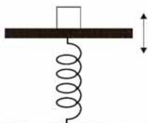
Figure 1.12 A particle on a horizontal plate executing SHM.
