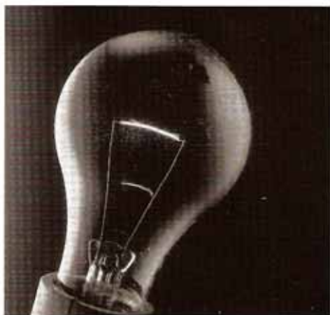
Figure 4.9 The metal filament in a light bulb glows as the current passes through it. It also feels warm. This shows that the bulb produces both heat and light.
