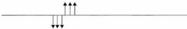
Figure 3.6 Parts of the rope are moving when the two pulses cancel each other out.
