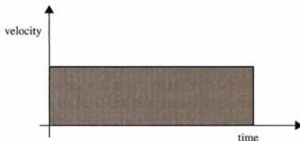
Figure 1.7 The area under the curve in a velocity-time graph gives the displacement change.
