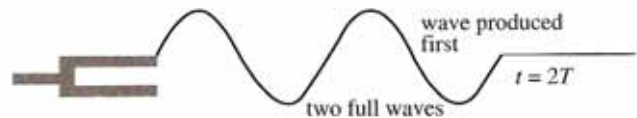
Figure 2.8 Two full waves are produced in sequence by the oscillating tuning fork.
