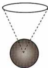
Figure E1.3 The axis of rotation of the earth precesses in space tracing out a cone. Now it points at the star Polaris. In the year AD 14 000 it will point at the star Vega. The period of precession is about 26 000 yr.
