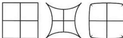
Figure G2.24 An example of distortion due to spherical aberration. The grid is distorted because the magnification varies as one moves away from the principal axis.
