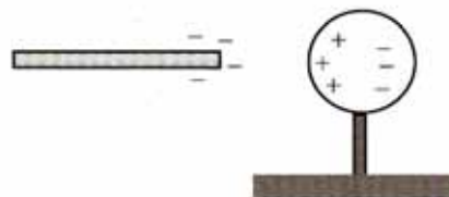
Figure 1.1 A negatively charged rod brought near to an insulated conductor forces electrons in the conductor to the side furthest from the rod.
