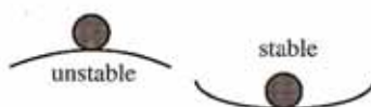
Figure 4.2 In unstable equilibrium the net force on the body is zero, but a small displacement results in motion away from the equilibrium position. In stable equilibrium, the motion is back towards the equilibrium position.
