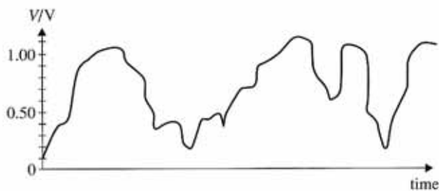
Figure F5.14 A very corrupt digital signal that must be reshaped.
