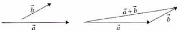
Figure 4.5 One of the vectors is shifted parallel to itself until its beginning point coincides with the end of the other vector. The sum is then the arrow that joins the only beginning point to the only end point.
