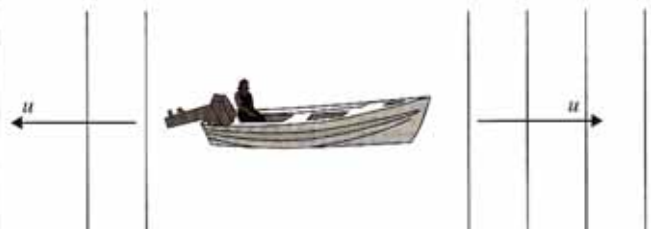
Figure H3.5 View from the boat at rest. The boat is at rest in the water and waves moving to the right and left move with the same speed relative to the boat. This velocity is u , the velocity of water waves relative to the water.
