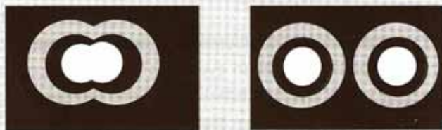
Figure 8.1 Diffraction limits our ability to distinguish two separate sources. In the first diagram the diffraction patterns have merged.
